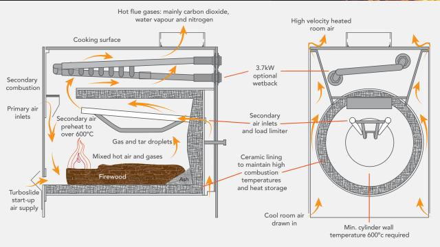
\*Please note: 12hr+ overnight burn claims are based on the Pyroclassic IV installed with our Eco Flue Kit with sufficient flue draw and fuelled with dry, hardwood logs.
